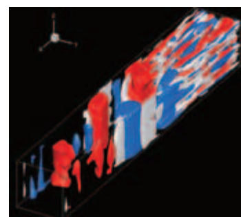
Eddies for a liquid metal turbulent flow in a square duct, to which a local magnetic field is applied
